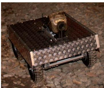
**Figure 49. The scout robot with the IR-image camera**
