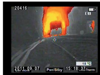
**Figure 46** From upstream the fire towards train at pulsations, low sensitivity mode, info Therm colouring
