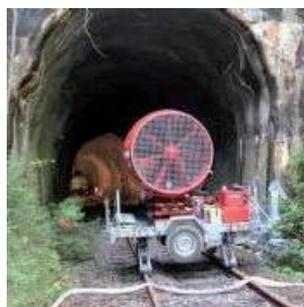
**Figure 50 Mobile high-flow ventilator**
