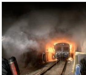
**Figure 53 Back-layering, test 2**
