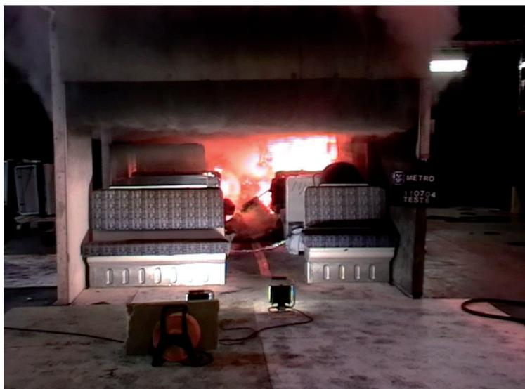
**Figure 2** Photo taken shortly after the fire starts to spread from the initial fire source with poured petrol in the right corner combined with combustible material on the walls, seats and luggage.
