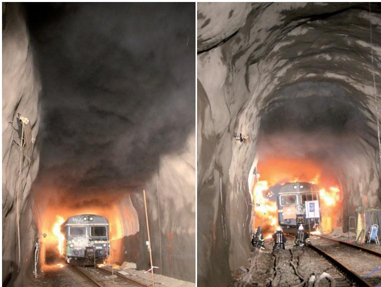
**Figure 10** Developed backlayering in test 2 (left) and large flames and progressing backlayering in test 3 (right).
