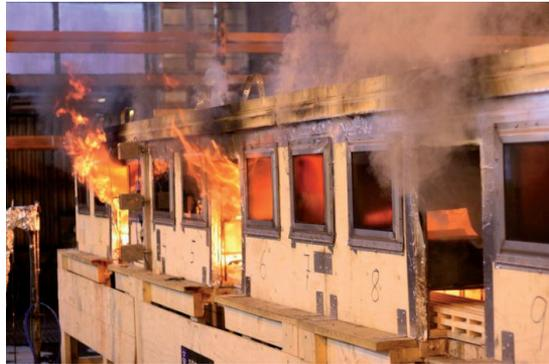
**Figure 1** A photo of the model scale experiments (1:3). The door to the left is door DR1 and the one in the middle is door DR2.
