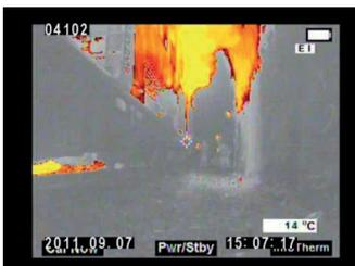
**Figure 43** Beside train pointing upstream fire, low sensitivity mode, info Therm Colouring
